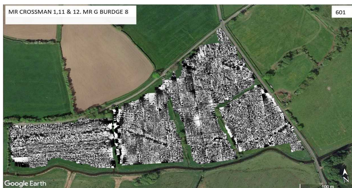
Fig 9: Black and white results from this survey (left) and adjacent gradiometry surveys on Google Earth image.
