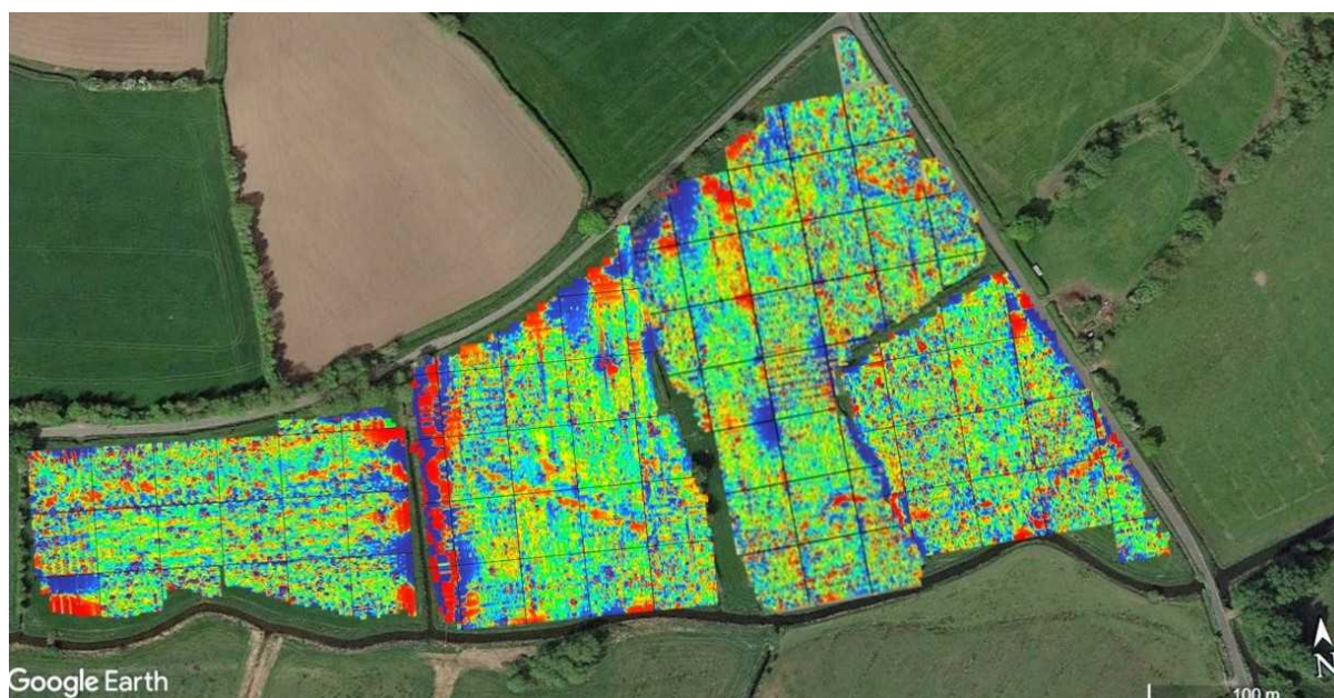
Fig 8: Colour results from this survey (left) and adjacent gradiometry surveys on Google Earth image.
