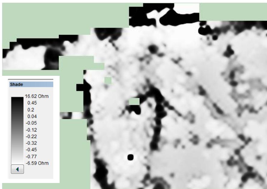
Fig 9: TerraSurveyor Shade image with filters as per Fig 8 plus High/Low Pass Filter
