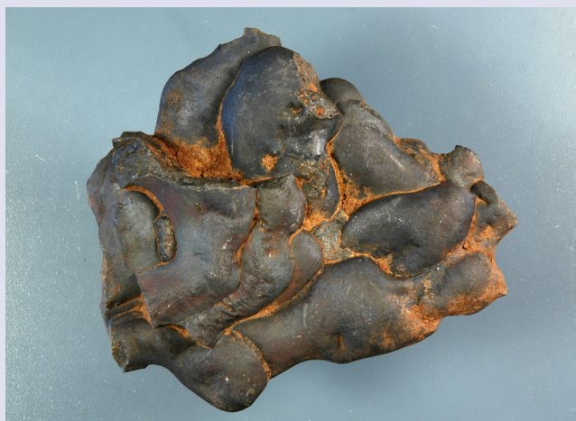
Two more examples of iron ore processing slag from Cobthorn, Congesbury. Photographs by John Wilcox.
