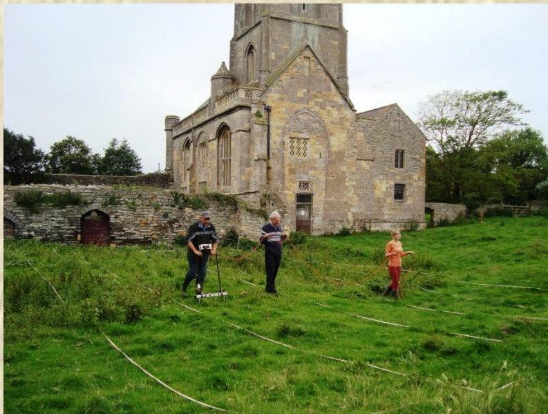
Using the resistivity meter at Woodspring Priory. The machine measures the resistance of the earth below it, which can detect walls or structures without excavating.
