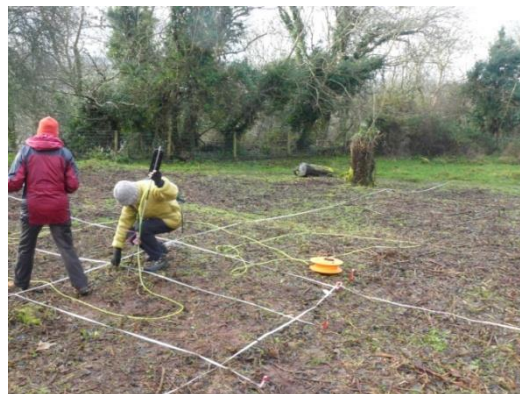
Figure 16. 'Square' shaped area in grid 1, identified on the ground. (Looking west). For feature A, a 7 x 6 m grid, was chosen, centred on the designated area (appendix 10). At intervals of 0.5m westerly, and 1m southerly, heights above, (+), and below,
