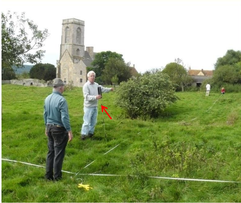
Fig 7. The electronic, hydrostatic level (arrow) in use; looking west.
