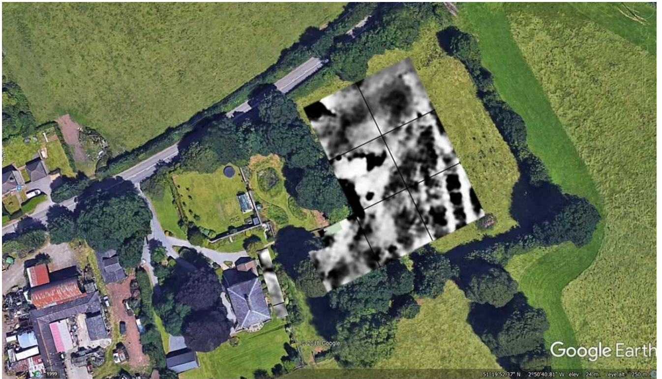
Fig 10: The resistivity results from site 1 & 2 (See arrow) superimposed on a Google Earth image
