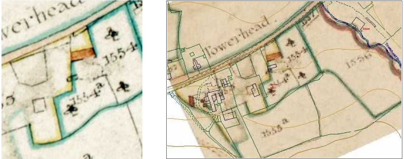
Fig 4: Towerhead House from the Tithe Map (1834, left) and (right) georeferenced to OS data. The match is not perfect, but the work of James Poole, the map's surveyor, seems tolerably accurate
